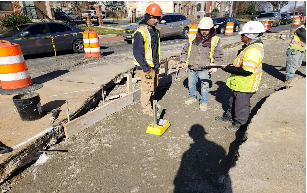
02/08/2020- Moisture Density Test for the bus pad at West side of New Jersey Ave. & N St. NW.
